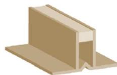
Special Profiles expansion joints allow the creation of large surfaces, avoiding cracks / over pressures deriving from the movements of the structures. Available in various heights, depending on the thickness of the floors, they are made by coextrusion of a rigid and robust PVC, and a soft and elastic transparent PVC. Thanks to this particular component, all unwanted vibrations and pressures on the floor are absorbed, avoiding breakage or lifting of the floors.
