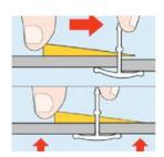
Remove the wedges hitting the tie-beams, once the glue is dried.
